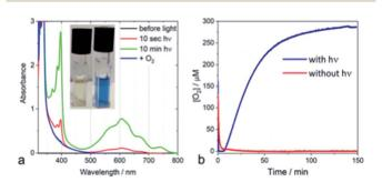
Fig. 2 (a) Spectral changes induced in an Ar-purged solution of nano-PDPB,  $100~\mu M~MV^{2+}$ , 10%~TEOA in MeCN by illumination with blue light and after aeration (inset: formation of the blue  $MV^{++}$  radical). (b) Time courses of oxygen evolution from water measured by a Clark electrode. Blue curve: with nano-PDPB (synthesized in mesophases) and red curve: no irradiation.
