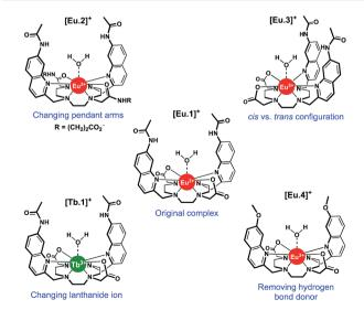
Fig. 1 Structures of Ln complexes [Eu.1-4]<sup>+</sup> and [Tb.1]<sup>+</sup>.
