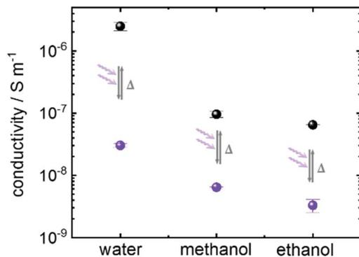
Fig. 4 Conductivity of water, ethanol and methanol in  $\text{Cu}_2(\text{SP-BPDC})_2(\text{dabco})$  SURMOF with the photoswitchable groups in the spiropyran form (black) and in the merocyanine form (violet). The experiments (Fig. 3 and S15†) are repeated three times. The average values and the standard deviations as error bars are shown here.
