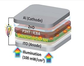
Fig. 11 BHJ PSC with the tool architecture: ITO/SPAN(SH)@GNP(X%) NH/P3HT; ICBA/ZnO/Al. Reproduced with permission from ref. 107. Copyright 2018 Elsevier.
