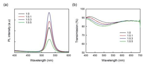
Fig. 5 (a) PL and (b) transmittance spectra of the CH<sub>3</sub>NH<sub>3</sub>PbBr<sub>3</sub> films covered on the PEDOT:PSS films doped with different GO amount.
