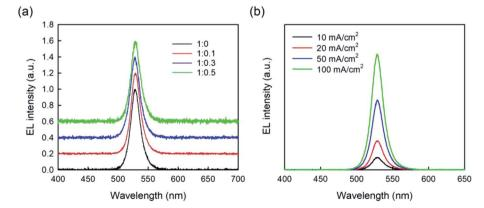
Fig. 8 (a) Normalized EL spectra of the PeLEDs with PEDOT:PSS HTLs doped with different GO amount tested at the current density of 50 mA cm<sup>-2</sup>. (b) EL spectra for the PeLED with the optimal PEDOT:PSS:GO (1:0.3) HTL tested by using different current densities.
