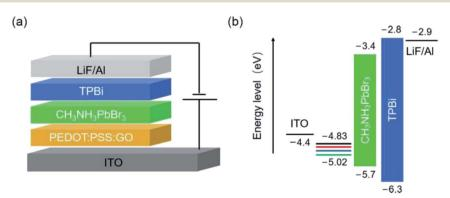
Fig. 1 (a) Schematic device structure of PeLEDs using GO doped PEDOT:PSS HTL. (b) Energy levels of individual layers for our PeLEDs.
