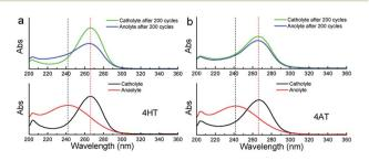
Fig. 7 Ultraviolet spectra of the anolyte and catholyte of the symmetric 4HT (a) and 4AT (b) RFBs, in 2 M KCl solution before and after 200 charge–discharge cycles.
