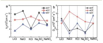
Fig. 4 Effect of supporting electrolytes (0.5 M) on electron transfer constant ( $k^0$ ) and diffusion coefficient (D).
