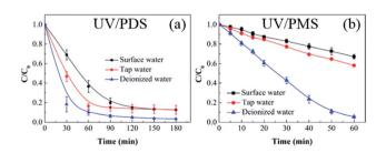
Fig. 7 HA removal from different water sources by UV/PDS (a) and UV/PMS (b). Conditions:  $[HA]_0 = 15 \text{ mg L}^{-1}$ ,  $[PDS]_0 = 3 \text{ mmol L}^{-1}$ ,  $[PMS]_0 = 1 \text{ mmol L}^{-1}$ ,  $pH_0 = 3.0$ , 7.4, and 7.8 for deionized water, surface water, and tap water, respectively.
