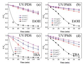
Fig. 4 Effects of radical scavengers on HA removal in UV/PDS (a and c) and UV/PMS (b and d). Conditions:  $[HA]_0=15~mg~L^{-1}$ ,  $[PDS]_0=3~mmol~L^{-1}$ ,  $[PMS]_0=1~mmol~L^{-1}$ ,  $pH_0=6~and~3~for~UV/PDS~and~UV/PMS$ , respectively.
