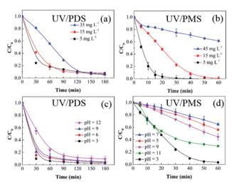
Fig. 3 Effects of the initial HA amount on HA removal in UV/PDS (a) and UV/PMS (b). Conditions:  $[HA]_0 = 5-45 \text{ mg L}^{-1}$ ,  $[PDS]_0 = 3 \text{ mmol L}^{-1}$ ,  $[PMS]_0 = 1 \text{ mmol L}^{-1}$ ,  $pH_0 = 6 \text{ and } 3 \text{ for UV/PDS and UV/PMS, respectively. Effects of the initial solution pH on HA removal in UV/PDS (c) and UV/PMS (d). Conditions: <math>[HA]_0 = 15 \text{ mg L}^{-1}$ ,  $[PDS]_0 = 3 \text{ mmol L}^{-1}$ ,  $[PMS]_0 = 1 \text{ mmol L}^{-1}$ ,  $pH_0 = 3-11$ .
