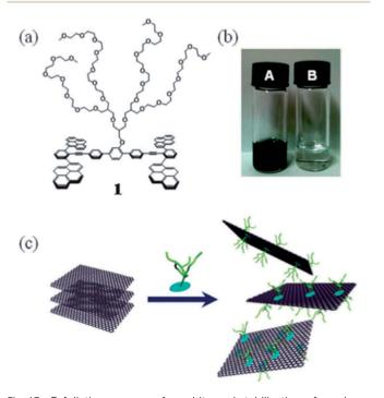
Fig. 13 Exfoliation process of graphite and stabilization of graphene though the  $\pi-\pi$  interaction with tetrapyrene derivative. This figure has been reproduced from ref. 91 with permission from *R. Soc. Chem.*, Copyright 2016.
