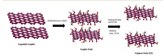
Fig. 4 Schematic synthesis of graphene oxide by the modified Hummers' method. This figure has been reproduced from ref. 53 with permission from *Chem. Mater.*, Copyright 1999.
