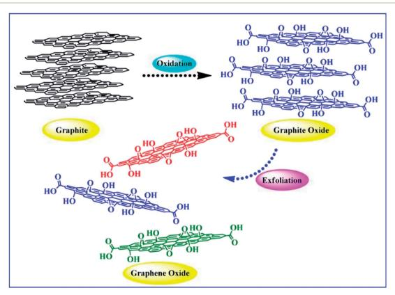
Fig. 3 Preparation of graphene oxide
