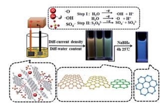
Fig. 1 A schema of the synthetic procedure of multi-color GQDs from the coke. Reprinted with permission.<sup>58</sup> Copyright 2018, Elsevier.
