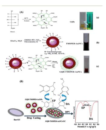
Fig. 10 A schema of the procurement process of (A) GQD-TMSPED-AuNCs nano-composites and (B) electro-chemically concurrent determination EP and DA. Reprinted with permission. Copyright 2019, Springer.
