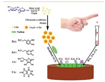
Fig. 8 A schema of the principle of electrochemical assay to detect dopamine based on cuprous the oxide-carbon dots/Nafion ( $Cu_2O-CDs/NF$ ) composite film. Reprinted with permission. <sup>129</sup> Copyright 2015, RSC.
