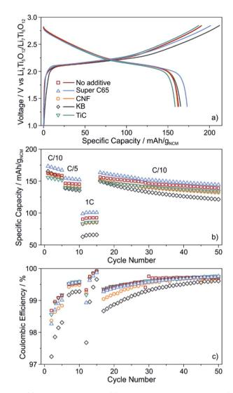
Fig. 3 (a) Initial voltage profile, (b) specific discharge capacity and (c) coulombic efficiency of SSB cells with and without conductive additive. All data are averaged from two independent cells.
