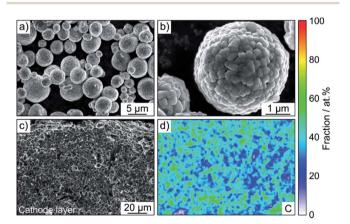
Fig. 2 (a and b) Top-view SEM images at different magnifications of the LiNbO $_3$ -coated NCM622 secondary particles. (c) Low-magnification cross-sectional SEM image of a pristine SSB cathode using Super C65 as conductive additive and (d) the corresponding elemental map of carbon.
