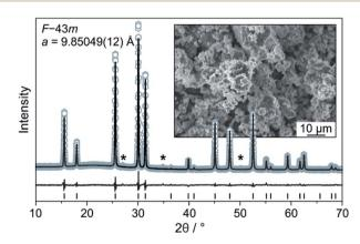
Fig. 1 Rietveld analysis of the XRD pattern for the Li<sub>6</sub>PS<sub>5</sub>Cl solid electrolyte. Asterisks denote impurities. The inset is a low-magnification SEM image of the as-prepared solid electrolyte powder.
