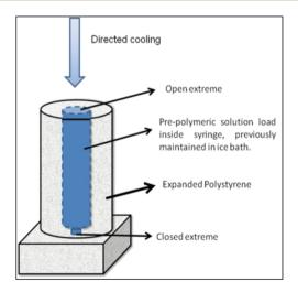
Scheme 1 Representation of the device by polymerization with directed cooling at  $-18\ ^{\circ}\text{C}.$
