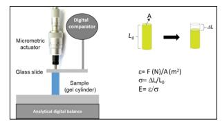
Scheme 2 Description of the device used to determine the elastic modulus
