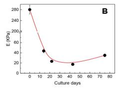
Fig. 3 (A) Maximum swelling capacity (% Sw(eq)) during several culture days. (B) Elastic modulus of the macroporous PNIPAM hydrogel cell seeding at different culture days measured by uniaxial compression in the culture condition.
