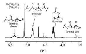
Fig. 9 Structure assignment of <sup>1</sup>H NMR peaks used for quantification of recycling products.
