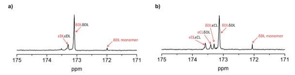
Fig. 8  $^{13}$ C NMR spectrum of (a) PδDL-co-20 $\epsilon$ DL show two single peaks corresponding to the homopolymer peaks, (b) PδDL-co-20 $\epsilon$ CL show four peaks corresponding to the homopolymer peaks as well as two dyad peaks representing the transitions between δDL and  $\epsilon$ CL.
