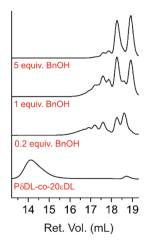
Fig. 10 CHCl $_3$  SEC elution diagram of the starting material P $\delta$ DL-co- $20\epsilon$ DL and the recycling product after 22 h at 150 °C with BnOH as external nucleophile and DPP as catalyst.
