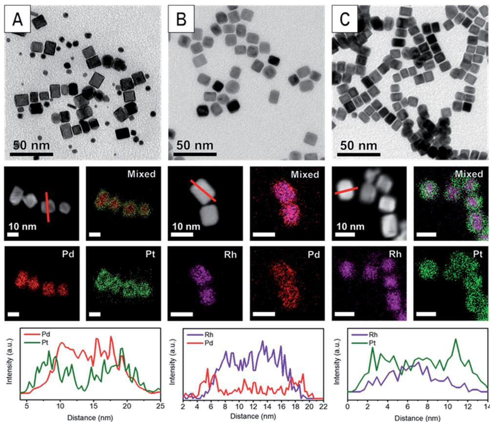
**Fig. 1** Characterization of (A) Pd@Pt, (B) Rh@Pd, and (C) Rh@Pt. The first row contains TEM images of each sample. The second and third row are STEM images and corresponding STEM-EDX elemental maps of the core@shell nanocrystals where green represents Pt, red Pd, and purple Rh. The last row is the line profiles indicated by the red line in the STEM image in the second row for each nanocrystal sample.
