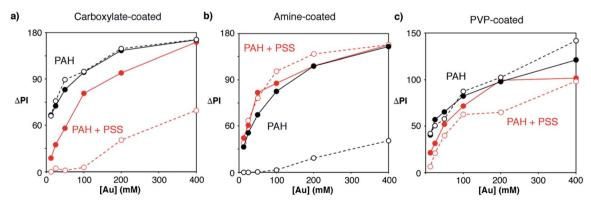
Fig. 4 Colorimetric signals ( $\Delta$ PI) generated by different concentrations of gold nanoprobes ([Au]) modified with avidin when the paper substrate was modified with PAH (black dots) or PAH and PSS (red dots), and biotinylated BSA (full dots) or non-biotinylated BSA (open dots). Nanoprobes modified with avidin were obtained using carboxylate-coated (a), amine-coated (b) or PVP-coated (c) nanoparticles.
