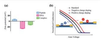
Fig. 6 (a) Zeta potential values of the CW peptide, DNA, and their complex. The electrostatic adsorption of the peptide and DNA occurred because of their opposite ZP and the formed complex had the same ZP as DNA, which hindered the continuous adsorption with DNA. (b) Illustration of the current change sensitive to charge doping. The negative charge doping induced a right shift of the characteristic curve, resulting in an enhanced current and *vice versa*.
