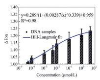
Fig. 5 The  $\Delta$ Ion signal responses to DNA concentrations from 5  $\times$   $10^{-5}$  to 5  $\mu$ mol L<sup>-1</sup>. The relationship between  $\Delta$ Ion and the DNA concentration could be fitted with the Hill–Langmuir model with a fitting correlation coefficient  $R^2$  of approximately 0.98. The error bars represent the standard error of the mean square root values from two independent experiments.
