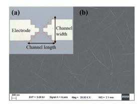
Fig. 2 (a) The optical microscope image of CNT TFT with Ti electrodes and CNTs; (b) the SEM image of the uniform CNT network.
