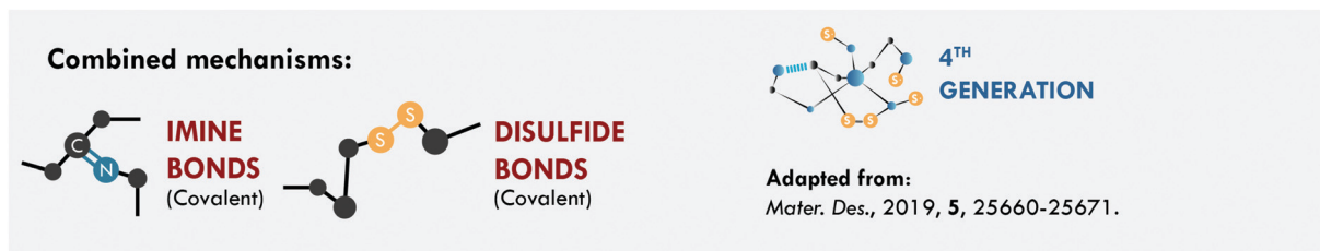
Fig. 9 Imine and disulfide metathesis in PU. 187 ©2019. Adapted with permission from Elsevier.
