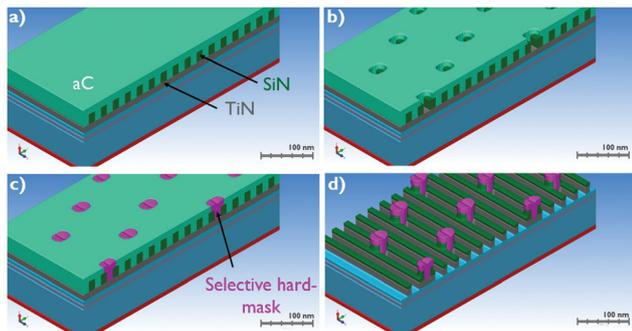
Fig. 1 (a–d) Proposed tone-inversion flow. Adopted by Briggs *et al.*<sup>2</sup>
