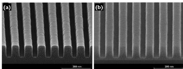
Fig. 5 Cross-sectional images of a-C lines after ICP He/H<sub>2</sub> plasma (a) before and (b) after SiO<sub>2</sub> hard-mask removal as measured *via* SEM.
