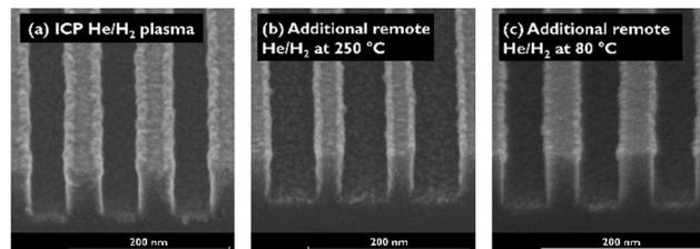
Fig. 6 Cross-sectional images of a-C lines after 100 cycles ALD of Ru at 275 °C as measured *via* SEM. (a) No pre-treatment, remote He/H<sub>2</sub> plasma pre-treatment at (b) 250 °C, and (c) 80 °C.
