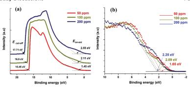
Fig. 4 (a) UPS spectra for the three different samples showing both cut-off and on-set values. (b) XPS valence band spectra showing the difference between VBM and Fermi level.
