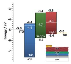
Fig. 6 Non-equilibrated band diagram for the PV device based on Si QDs as active layers,  $Cu_2O$  QDs as an electron blocking layer, a  $TiO_2$  film hole blocking layer and corresponding contacts. Inset: diagram of the layer structure of the device.
