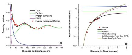
Fig. 2 (a) Fluorescence damping rate of a mixed dye LB monolayer vs. distance to bulk silicon (after ref. 39). (b) Normalised fluorescence lifetime of various chain length diol linked protoporphyrin silicon surfaces (after ref. 24).
