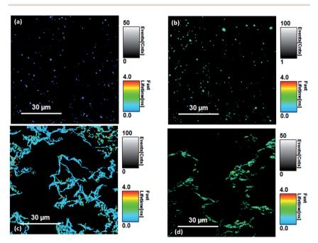
Fig. 5 Fluorescence lifetime imaging (FLIM) scans of (a) the Si-Vinyl-Pe surface, (b) the Si-Allyl-Pe surface, (c) the Pe-LB1 Si surface and (d) the Pe-LB2 Si surfaces.
