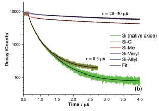
Fig. 4 (a) Emission spectra of various silicon treated surfaces; a clean silicon surface with native oxide present, Si (native oxide), a chlorinated silicon surface (Si-Cl), a methyl terminated silicon surface (Si-Me), a vinyl terminated silicon surface (Si-Vinyl) and an allyl terminated silicon surface (Si-Allyl). (b) Emission decay curves from the functionalised silicon surfaces at the maximum emission.
