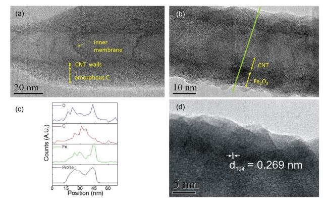
Fig. 3 High resolution TEM analysis of (a) pristine utCNTs. CNT walls, inner membranes and the amorphous C layer are indicated by arrows. (b) 6 nm  $Fe_2O_3$ @wpCNTs; (c) elemental line profile of O, C and Fe acquired along the green line marked in (b). (d) High resolution TEM of the  $Fe_2O_3$  coating on wpCNTs revealing an interplanar spacing of  $d \sim 0.269$  nm for iron oxide.
