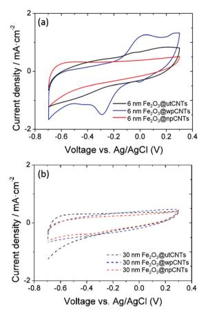
Fig. 6 Areal capacitance of carbon nanotubes with and without plasma treatment, covered with 6 and 30 nm thickness ALD-iron oxide at a 50 mV s<sup>-1</sup> scan rate.
