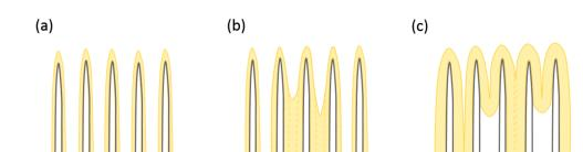
Fig. 2 Illustration of different ALD coatings of  $Fe_2O_3$  on the CNT surface: (a) conformal coating; (b) partial conformal coating and partial CNT aggregation; (c) thicker and non-conformal coating on CNTs.
