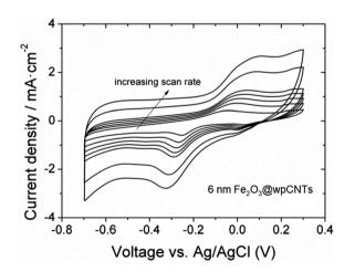
Fig. 7 Cyclic voltammograms of 6 nm Fe<sub>2</sub>O<sub>3</sub>@wpCNTs at scan rates from 10 to 150 mV s<sup>-1</sup>.
