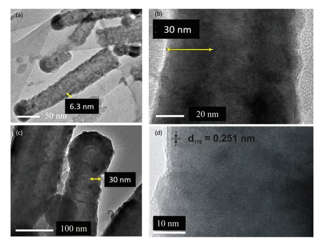
Fig. 4 (a) TEM images of 6 nm Fe<sub>2</sub>O<sub>3</sub>@npCNTs and (b) 30 nm Fe<sub>2</sub>O<sub>3</sub>@utCNTs and (c) and (d) high resolution TEM images of 30 nm Fe<sub>2</sub>O<sub>3</sub>@wpCNTs.
