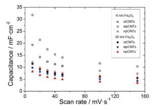
Areal capacitances of different nanocomposites versus scan rates.
