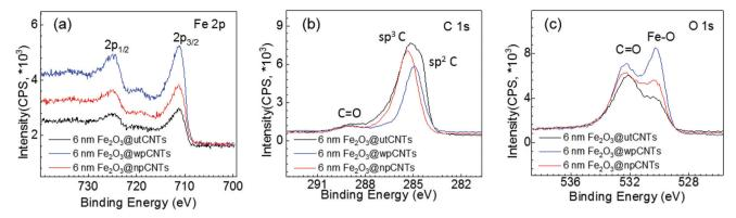
Fig. 5 (a) High-resolution Fe 2p spectra; (b) C 1s spectra and (c) O 1s spectra of 6 nm  $Fe_2O_3$ @CNTs.
