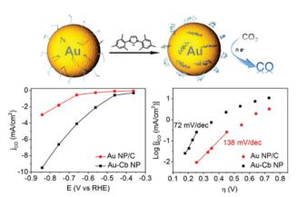
Fig. 35 Schematic illustration of NHC-carbene functionalized Au NPs for  $CO_2RR$  to CO. Partial current density and Tafel plot for CO production for Au–Cb NP and Au NP/C. Reproduced with permission from ref. 454. Copyright 2016 American Chemical Society.
