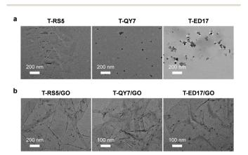
Fig. 2 Transmission electron microscopic images of (a) T-RS5, T-QY7 and T-ED17 (10  $\mu$ M), and (b) T-RS5/GO, T-QY7/GO and T-ED17/GO (peptide/GO = 10  $\mu$ M/40  $\mu$ g mL<sup>-1</sup>).
