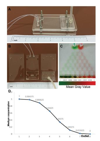
Fig. 2 Manufacture and characterization of the microfluidic chip. (A) The integral structure of the microfluidic chip; (B) the three layers of the microfluidic chip; (C) the tree-like flow pattern in the microfluidic chip for the generation of a concentration gradient, and illustration with two dyes with a red and a green color; and (D) the medium concentration gradient created in the culture chamber.
