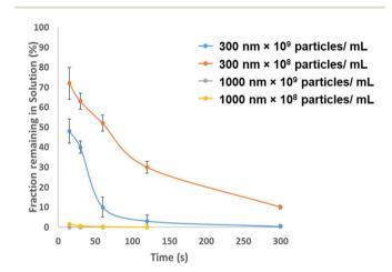
Fig. 5 Separation efficiencies for 300 nm and 1000 nm particles are different concentrations, error bars shows the st. dev of triplicate experiments. Plotted are bars for the 1 µm particles but the variation in measurements was low and is not visible on the graph.
