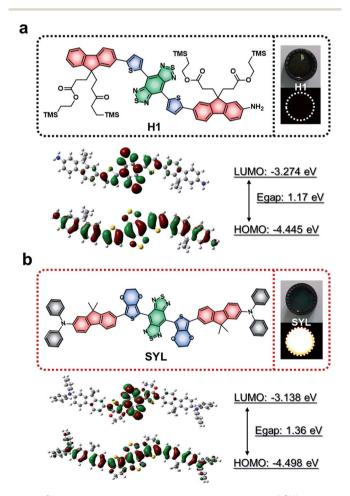
Fig. 2 Chemical structures and electronic properties of SYL and the previously reported NIR-II dye H1; (a) Frontier orbitals of H1, its associated energies (DFT using B3LYP Gaussian 09), and NIR-II fluorescence signals. (b) Chemical structures, NIR-II fluorescence signals and Frontier orbitals with associated energies of the novel NIR-II dye SYL.
