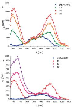
Fig. 5 Comparison of the 2PA spectra of (a) vinyl derivatives 13–15 and DEAC450 in DMSO; (b) dipolar compounds 14, 17, 19 and DEAC450 in DMSO.
