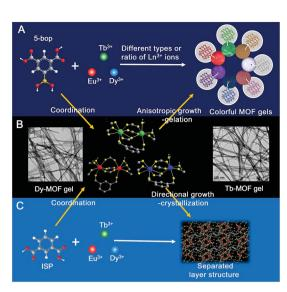
Fig. 1 (A) The selection of different types and ratios of  ${\rm Ln}^{3+}$  ions for the formation of MOF gels with different colors. (B) The formation of Tb- and Dy-MOF gels because of their different coordination environments compared to that of  ${\rm Eu}^{3+}$ . (C) Separated layer structure revealed from single crystal results for the formation of nanoribbons, which entangle together to form MOF gels.
