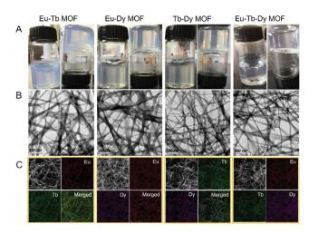
Fig. 5 (A) Photos and (B) TEM images of Eu–Tb, Eu–Dy, Tb–Dy, and Eu–Tb–Dy mixed-metal MOFs prepared with 5-bop as the ligand and 0.1 mmol mixed-metal precursors with metal ratios of 1:1 or 1:1:1 in 10 mL of DMF/H<sub>2</sub>O at 120 °C under atmospheric pressure. (C) Scanning transmission electron microscopy images and energy-dispersive X-ray elemental mapping of the mixed-metal MOF gels.
