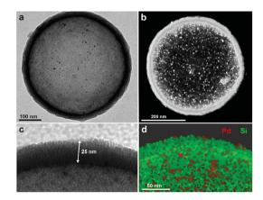
Fig. 2 Characterization of Pd-Cap1. (a) Representative TEM image (500 nm diameter); (b) STEM image; (c) zoom-in view showing the vertically oriented mesopores in the silica shell with a thickness of 25 nm; (d) XEDS mapping showing the elemental distribution of Pd
