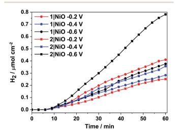
Fig. 8 Cumulative photoelectrocatalytic  $H_2$  production by 1|NiO and 2|NiO during the chronoamperometry measurements at different  $E_{\rm appl}$  (Fig. 7 and S3 in the ESI†). Chopped light illumination was applied during the first 10 min followed by constant light illumination until the end of the measurement (AM1.5, 100 mW cm<sup>-2</sup>).
