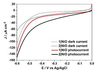
Fig. 6 Linear sweep voltammograms of 1|NiO and 2|NiO immersed in aqueous 0.1 M KCl electrolyte (pH 3). The potential was sweet from  $E_{\rm appl} = 0$  to -0.6 V vs. Ag/AgCl (3.0 M NaCl) in the dark and under simulated light illumination (AM1.5, 100 mW cm<sup>-2</sup>).
