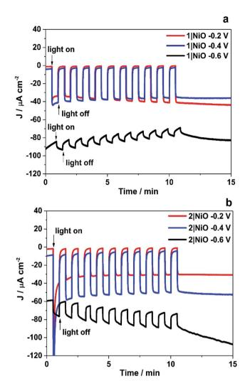
Fig. 7 Chronoamperometry measurements of 1|NiO (a) and 2|NiO (b) immersed in pH 3 buffer containing 0.1 M potassium hydrogen phthalate.  $E_{appl} = -0.2$  V, -0.4 V and -0.6 V vs. Ag/AgCl (3.0 M NaCl). Chopped light illumination was applied with 30 s intervals (10 cycles of dark current/photocurrent).
