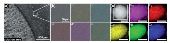
Fig. 5 Scanning electron microscope image (secondary electrons) of an ablation target near the border of an ablation area (a), elemental maps of Co, Cr, Fe, Mn, and Ni obtained by energy dispersive X-ray spectroscopy of a non-ablated target area (b), and scanning transmission electron microscopy image and elemental maps of Co, Cr, Fe, Mn, and Ni for a single nanoparticle (c). In (a), the laser ablation area is located on the left side of the image. In (c), all scale bars represent 25 nm.
