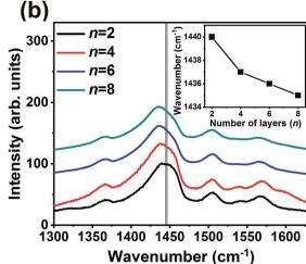
Fig. 3 The Raman spectra of single layer-PEDOT:PSS thin films as a function of spin speed and (b) PEDOT:PSS/PANI-CSA ML thin films with respect to the number of layers. The insets of (a) and (b) show the corresponding variations of the peak of the  $C_{\alpha} = C_{\beta}$  vibrations.
