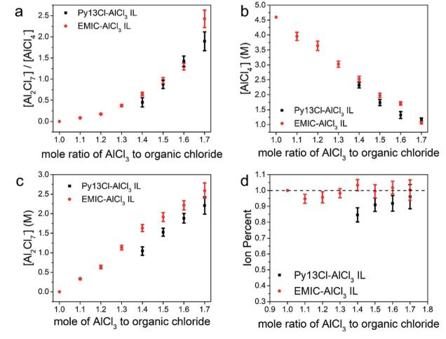
Fig. 4 Species concentrations and ion percent comparison between Py13Cl–AlCl<sub>3</sub> and EMIC-AlCl<sub>3</sub> ionic liquids (a) [Dimer] to [Monomer] ratios comparison between these two ionic liquids, (b) monomer concentration comparison between these two ionic liquids, (c) dimer concentration comparison between these two ionic liquids, (d) ion percent comparison between these two ionic liquids.
