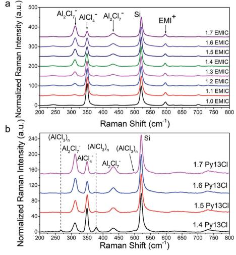
Fig. 2 Raman spectra of Py13Cl-AlCl<sub>3</sub> and EMIC-AlCl<sub>3</sub> ionic liquid, normalized by the Si wafer peak at around 520 cm<sup>-1</sup>. (a) Raman spectra of with species assignment to major peaks.
