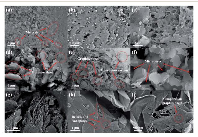
Fig. 3 SEM images of lignite, impregnated lignite and synthetic graphite samples: (a) lignite; (b) and (c) impregnated lignite; (d) – (f) LG-2700; (g) – (i) ILG-2700.
