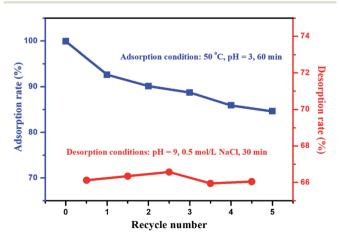
Effect of the recycle number on adsorption and desorption.
