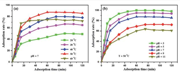
Fig. 7 Influence of adsorption temperature (a) and pH value (b) on the adsorption rate of the methyl orange solution.
