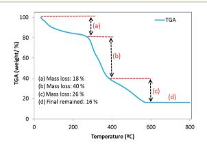
Fig. 8 Thermogravimetric analysis (TGA) plot of the fabricated biomagnetic membrane capsules (BMMCs). (Reproduced from Ali *et al.*<sup>24</sup> Copyright@2019, with permission from Elsevier Ltd.)
