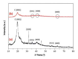
Fig. 4 Powder X-ray diffraction patterns of (a) PVA–SA–PMNPs and (b) the prepared bio-magnetic membrane capsules (BMMCs) after reaction with primary and secondary cross-linking agents (displaying the amorphous carbon and magnetite structures). (Reproduced from Ali *et al.*<sup>24</sup> Copyright@2019, with permission from Elsevier Ltd.)
