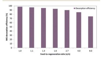
Fig. 14 Effect of different feed-to-regeneration ratios (v/v) on the desorption efficiency of malachite green (MG) dye (water as regeneration solution; adsorbent dosage = 0.02 g L<sup>-1</sup>, MG initial concentration ( $C_0$ ) = 25 mg L<sup>-1</sup>; replication = 3; standard deviation:  $\pm$  1.59).
