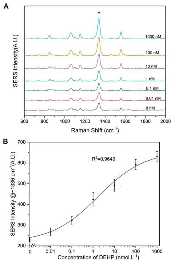
Fig. 7 (A) Response of the aptasensor to different concentrations of DEHP in  $0.1\text{ M}$  pH  $7.4$  PBS. (B) Average of SERS peak intensity at  $\sim 1336\text{ cm}^{-1}$  as a function of DEHP concentration. Error bar represents standard deviation ( $n = 3$ ).
