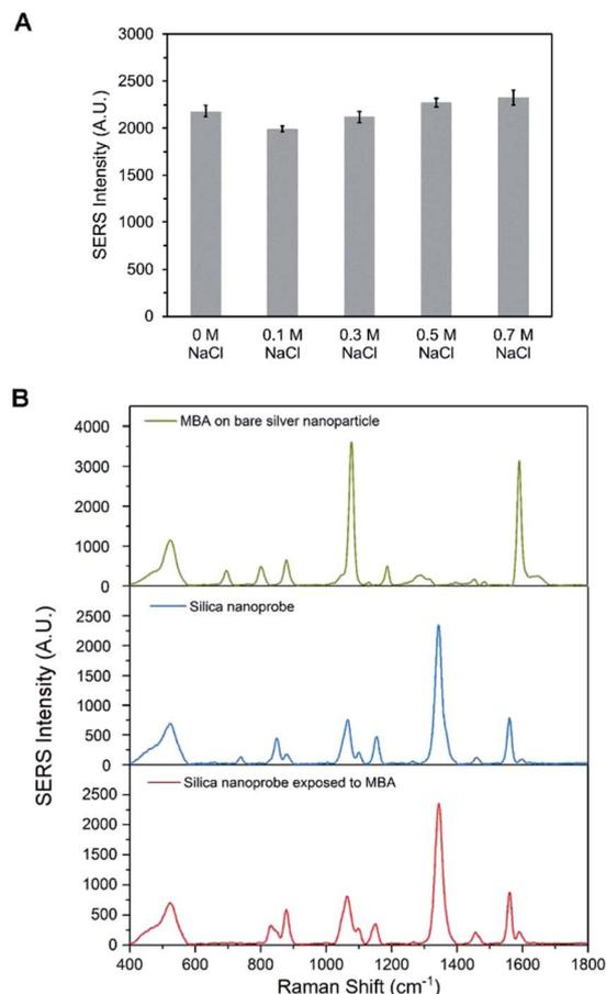
Fig. 6 Stability of the DEHP functionalized SERS silica particles. (A) SERS intensity at  $1336\text{ cm}^{-1}$  of the SERS silica particles after 1 h exposure to PBS ( $0.1\text{ M}$ , pH 7.4) with  $0.1\text{ M}$ ,  $0.2\text{ M}$ ,  $0.5\text{ M}$ , and  $0.7\text{ M}$  NaCl. (B) SERS spectra of Ag nanoparticles after 1 h exposure to  $0.5\text{ mM}$  4-MBA, and SERS silica particles after no exposure and exposure to  $0.5\text{ mM}$  4-MBA.
