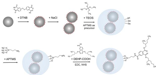
Fig. 1 Schematic diagram of the process to fabricate the DEHP modified SERS silica particles: first, DTNB was functionalized on AgNPs. Then, NaCl was introduced to form clusters of AgNPs. The AgNCs were then coated with a silica shell. Subsequently, AgNCs-SiO<sub>2</sub> was functionalized with APTMS to create a surface with primary amines. Finally, DEHP-COOH was immobilized on the AgNCs-SiO<sub>2</sub>-NH<sub>2</sub> by an amide bond using EDC/NHS chemistry.
