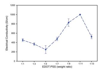
Fig. 8 Electrical conductivity of PEDOT:PSS at the EDOT:  $Na_2S_2O_8$  mole ratio of 1:1 and at various EDOT: PSS weight ratios.
