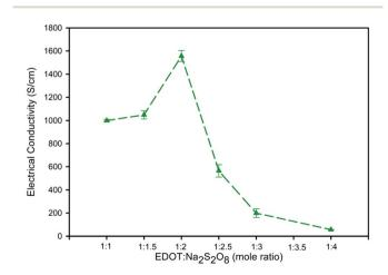
Fig. 9 Electrical conductivity of PEDOT: PSS at the EDOT : PSS weight ratio of 1 : 11 and at various EDOT :  $Na_2S_2O_8$  mole ratios.
