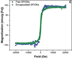
Fig. 1 Characterization of free and encapsulated SPIONs by transmission electron microscopy (TEM) and superconducting quantum interference device (SQUID). TEM of free and encapsulated SPIONs is presented in (a) and (b), respectively. SQUID magnetisation curves are shown in (c).
