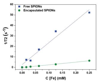
Effect of encapsulation of SPIONs on the solution relaxivity. The water relaxation rates are plotted against the concentrations of particles (in terms of Fe content).
