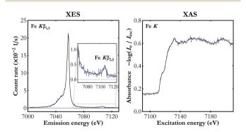
Fig. 3 The simultaneous Fe Kβ XES and Fe K-edge XAS measurement for two acquisition times: 2 hours (blue line) and 20 hours (black line).
