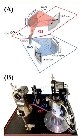
Fig. 1 (A) Conceptual model of the X-ray setup. (B) View of the developed double von Hámos spectrometer. Not shown is an additional lead shielding fixed to the XES detector during measurements which allowed the contribution of the scattered photons to be significantly reduced.
