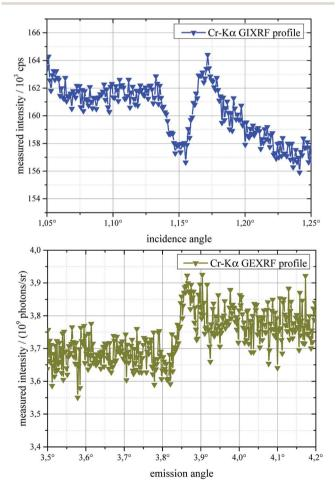
Fig. 7 GI- (top) and SF-GEXRF (bottom) of a chromium–scandium multilayer with a period thickness of 1.7 nm. The GIXRF scan is performed with an angular resolution of 0.001° and each point is measured for 5 seconds. In the SF-GEXRF measurement 10 000 CCD frames are recorded with an exposure time of 3 seconds.
