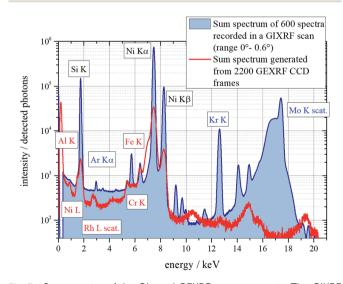
Fig. 3 Sum spectra of the GI- and GEXRF measurements. The GIXRF sum spectrum (blue) is generated from 600 individual spectra recorded during a scan in the range 0-0.6° with a step size of 0.001°. For the GEXRF sum spectrum (red) 2200 CCD frames were evaluated. The elemental labels are indicated in red if the element can only be found in the GEXRF sum spectrum, blue if solely the GIXRF spectrum shows it, and black when the element is present in both sum spectra.
