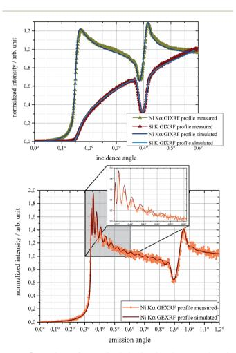
Fig. 5 Comparison of normalized simulated and measured angle resolved XRF profiles of the NiC multilayer. For GIXRF (top) the profiles of the fluorescence lines of Ni Kα (green) and Si K (red) are evaluated, and for SF-GEXRF (bottom) only those of Ni Ka. A magnified image of the angular region from 0.3° up to 0.6° of the SF-GEXRF profile is shown to emphasize the overlap of the fine interference structures of the profile
