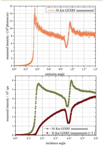
Fig. 4 Angle resolved elemental profiles of the NiC multilayer. For the SF-GEXRF measurements (top) only the Ni K $\alpha$  fluorescence line profile is shown. An angular resolution of 0.005° enables the discrimination of fine interference structures not visible in the respective GIXRF profile (bottom). The GIXRF profiles of the Ni Kα (green) and Si K (red) fluorescence lines are shown. The profile of silicon is multiplied by a factor 5 to display it in one plot with nickel
