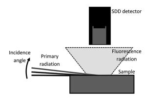
Fig. 1 Schematic representation of the GIXRF measurement geometry. The incident beam of the primary radiation on the sample is varied by either changing the position of the X-ray source or tilting the sample relative to the beam. The fluorescence radiation from the sample is detected in a short distance above the surface with an SDD detector.
