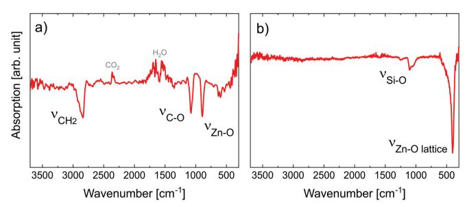
Fig. 2 FT-IR spectra of (a) 50 nm-thick MLD zincone layer right after deposition and (b) 27 nm-thick calcined MLD-derived ZnO treated up to  $600 \, ^{\circ}$ C.  $\nu$  symbols refer to the stretching modes.
