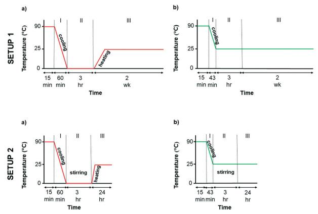
Fig. 2 Diagrams illustrate the different temperature profiles used in this study. Setup 1 is quiescent conditions and setup 2 is stirring conditions, each using controlled cooling to (a) 0 °C, and (b) 25 °C
