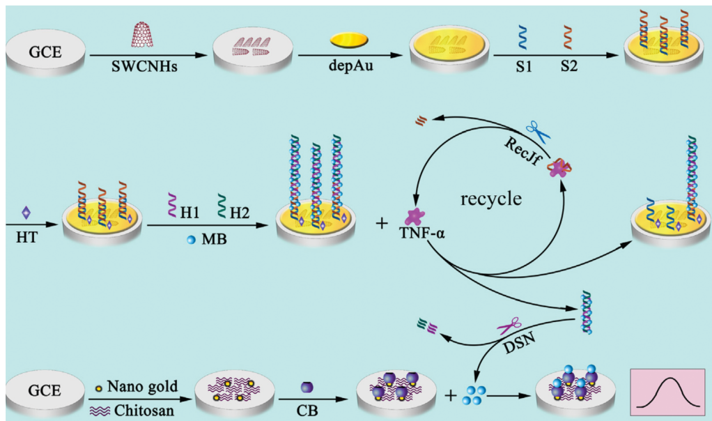
Fig. 7 Schematic illustration of the HCR and target recycling enhanced aptasensor for TNF- \alpha with host-guest interactions for signal probe collection. Reproduced from ref. 121 with permission.
