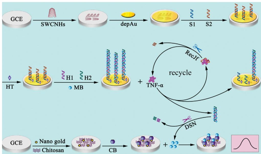
Fig. 7 Schematic illustration of the HCR and target recycling enhanced aptasensor for TNF- \alpha with host-guest interactions for signal probe collection. Reproduced from ref. 121 with permission.
