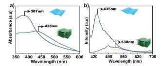
Fig. 4 UV-vis (a) and emission (b) spectra of bulk TTA-DFP COFs (green line) and exfoliated TTA-DFP CONs (blue line) dispersed in water at room temperature,  $\lambda_{\rm ex}=375$  nm.
