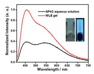
Fig. 7 PL emission spectra of the WLE hydrogel ( $\sim$ 2 wt%) and its adopted NP4C aqueous solution excited at 400 nm, [NP4C] = 0.1 mM, and 25 °C. Inset: photographs of the WLE hydrogel in daylight and 365 nm UV light, respectively.
