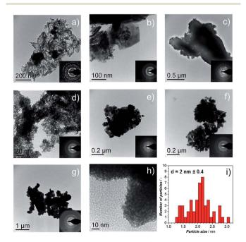
Fig. 3 TEM images of catalysts (a) Ir-black; (b) Ir-nano  $H_2O$ ; (c) Ir-nano 91.5; (d) Ir-nano 99.5\CTAB; (e) Ir-nano 99.5; (f) Ir-nano 99.8; and (g), (h) Ir-nano 99.8-P; the insets show the electron diffraction pattern from the synthesized materials showing the (111), (002), (022), (311), and (222) reflections of metallic Ir. (i) Histogram of Ir-nano 99.8-P.
