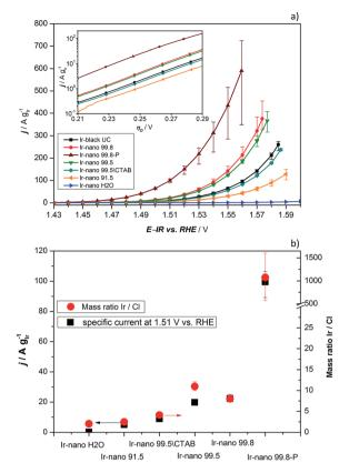
Fig. 5 (a) OER activity of all compared catalysts. The scanning rate, temperature and rotation speed are 5 mV s $^{-1}$ , 25 °C, and 2300 rpm, respectively. The measurements were performed in 0.5 M H $_2$ SO $_4$  and Ar-saturated solution; the inset shows the data as Tafel plots; (b) specific current density at 1.51 V vs. RHE measured under the same experimental conditions. The right axis indicates the Ir/Cl mass ratio recorded by EDX.
