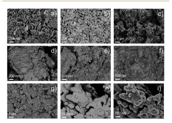
Fig. 2 SEM images from the secondary and back-scattered electron signals (SE, BSE) of catalysts (a) SE Ir-black and (b) BSE Ir-black; (c) SE Ir-nano  $H_2O$ ; (d) BSE Ir-nano 91.5; (e) BSE Ir-nano 99.5\CTAB; (f) BSE Ir-nano 99.5; (g) BSE Ir-nano 99.8; and (h) BSE Ir-nano 99.8-P, (i) SE Ir-nano 99.8-P.
