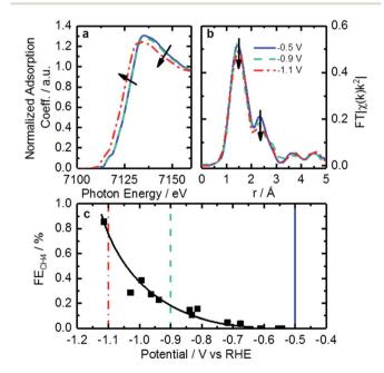
Fig. 7 Fe K-edge XANES (a) and EXAFS (b) spectra taken under *operando* conditions in  $CO_2$ -saturated 0.1 M KHCO $_3$  at -0.5 V (solid blue curves), -0.9 V (dashed green curves) and -1.1 V (red dot-dashed curves) vs. RHE. (c) Faradaic efficiency to  $CH_4$  varying with potential. Lines are added to indicate points representative of spectra in (a) and (b).
