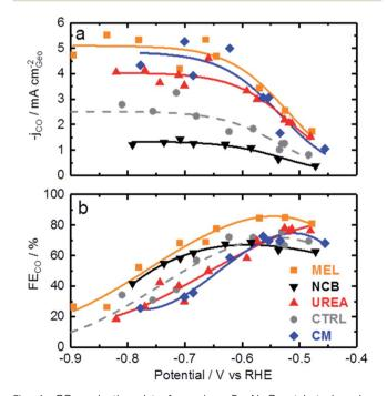
Fig. 4 CO<sub>2</sub> reduction data for various Fe-N-C catalysts based on different secondary nitrogen precursors: (a) CO generation rate, (b) faradaic efficiency towards CO production. Experimental conditions: CO2 saturated 0.1 M KHCO<sub>3</sub>, catalyst loading: 0.75 mg cm<sup>-2</sup> on glassy carbon.
