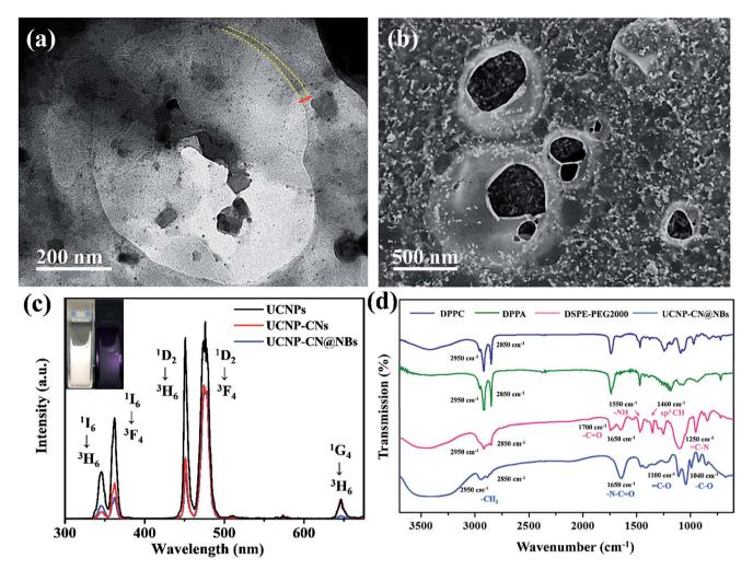
Fig. 3 (a) TEM and (b) SEM images of UCNP-CN@NBs. (c) UV-vis and photoluminescence spectra of UCNP-CN@NBs. UCNP-CN@NBs were irradiated by a 808 nm laser at 0.5 W cm<sup>-2</sup>. (d) FTIR spectra of UCNP-CN@NBs.
