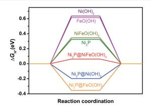
Fig. 4 Free energy of H\* adsorption on different catalysts by DFT calculations.
