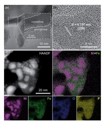
Fig. 2 (a) TEM image, (b) HRTEM image, (c) HAADF-STEM image and EDS elemental mapping images for the  $Ni_2P@FePO_x$  sample.
