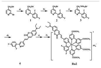
Scheme 2 The synthetic route of complex Ru2. (a) 2,4-Difluor-ophenylboronic acid, Pd(PPh $_3$ ) $_4$ , Na $_2$ CO $_3$ , toluene, reflux, 12 h; (b) 48% HBr, reflux, 6 h; (c) PPh $_3$ , toluene, reflux, 5 h; (d) 7-dieth-ylaminocoumarin-3-aldehyde, K $_2$ CO $_3$ , THF, 0 °C; (e) [Ru(cycme)Cl $_2$ ] $_2$ , CH $_3$ CN, 50 °C, 24 h; (f) 4,4'-dimethylester-2,2'-bipyridine, CH $_3$ OH, reflux, 5 h.
