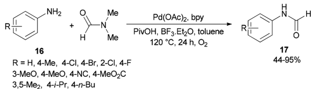
Scheme 6 Transamidation of aniline derivatives 16 with dimethylformamide.
